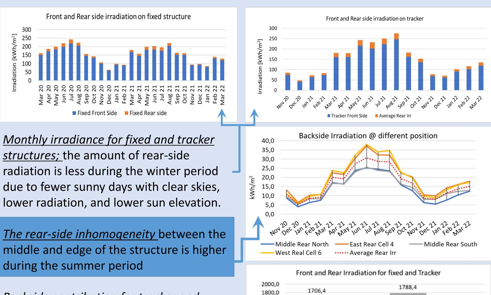
Backside contribution for tracker and fixed bench (1 Year): 10.4% for the tracker and 8.4% for the fixed structure; the effective irradiation (rear + front) on the tracking bench is 6,72% higher compared to fixed one
