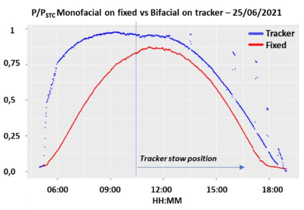
Power curves of the tracker in *Stow*Position: the power curve of the tracker takes the typical shape of a fixed system.
