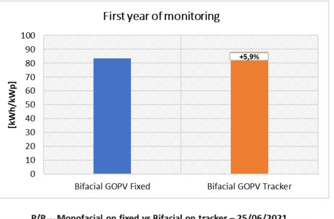
GOPV bifacial (tracker) vs. GOPV bifacial (fixed) -> Tracker energy gain +5,9%(based on only 12 days selected over the year); the expected, model-based was ~7%
