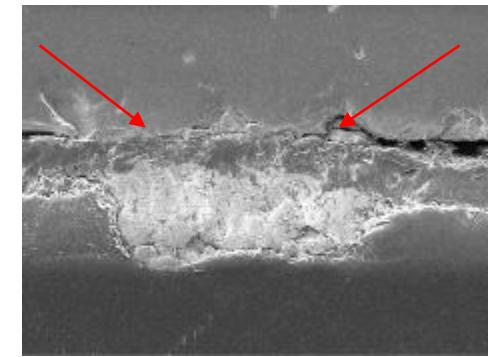
Resin between fingers and cell → previously delaminated
