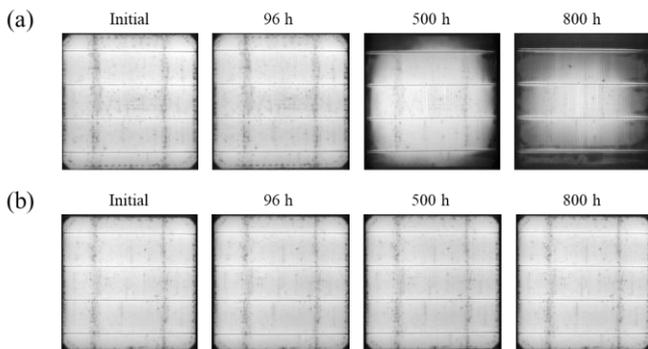
**Figure 4.** EL images of (a) G/G and (b) G/G – ES mini-module before and after 1000 h of PID test at 85°C/85% RH/-1000 V. For the G/G mini-modules degradation starts at the edges of the module after 500 h of test, gradually expanding the inactive area. On the other hand, G/G – ES module configuration prevents degradation by PID even when EVA is used.
