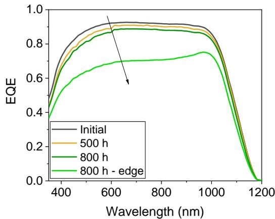
**Figure 3.** EQE measurements of a G/G mini-module subjected to PID test at 85°C/85% RH/-1000 V for up to 800h. Measurements were performed at the center and edges of the mini-module. The degradation at short wavelengths of the edges is more pronounced than at the centers.
