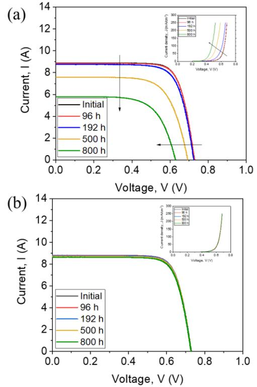
**Figure 2.** One-sun IV curves of (a) G/G and (b) G/G – ES mini-modules with EVA subjected to PID test at 85°C/85% RH/-1000 V for up to 800 h. Dark IV curves of the same sample are shown in the inset due to space constraints. We observe that both the one-sun and dark I-V curves remain stable in the case of the G/G – ES mini-module, whereas there is a gradual degradation for the mini-modules without an edge seal.
