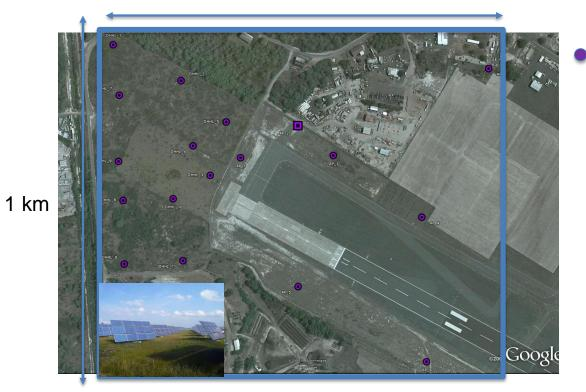
NREL Solar Measurement grid at Oahu : 1-s solar measurements from 17 photodiode pyranometers (Data available at: <u>www.nrel.gov/midc/oahu\_archive</u>)
