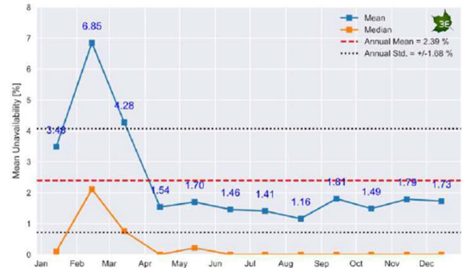
Figure 14: Statistical indicators of mean monthly unavailability of 533 PV plants in 2019 (majority installed in Belgium, Germany and Switzerland)
