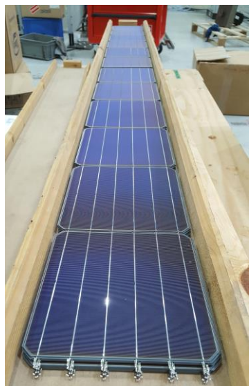
6 ECA-bonded ribbons interconnected cells Strings fabricated @ MASS
