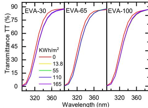
**Figure 4:** UV-Vis-NIR spectra of the G/G samples encapsulated with EVA-30, EVA-65, and EVA-100
