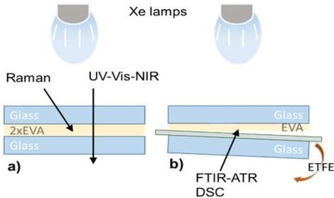
**Figure 1:** cross-sectional sketch of the sample structures used to characterise the encapsulant properties changes during aging.
