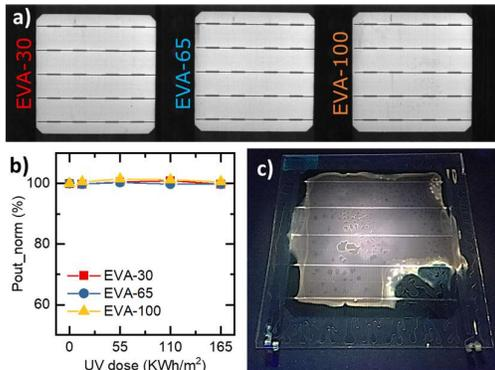
**Figure 3:** (a) electroluminescence images of 1 cell mini-modules after 165 kWh/m<sup>2</sup> of UV dose exposure; (b) power output (Pout) of modules during UV aging; (c) fluorescence images of EVA-100 after 165 kWh/m<sup>2</sup> of UV dose.
