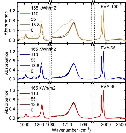
**Figure 6:** FTIR-ATR spectra recorded during UV aging for the different samples. Measurements are performed on *extracted-EVA* sample type.
