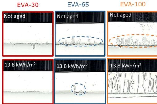
**Figure 2:** Visual inspection of 1 cell mini-module edges encapsulated with EVA-30, EVA-65, and EVA-100. The images on the top row correspond to unaged samples; Images on the bottom row have been taken after 13.8 kWh/m<sup>2</sup> of UV dose exposure.
