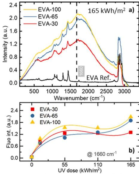
**Figure 5:** a) Raman spectra of the G/G samples collected after a UV dose of 165 kWh/m<sup>2</sup> (black curve corresponds to the unaged EVA); b) Fluorescence peak (at 1660 cm<sup>-1</sup>) intensity trend during UV aging.
