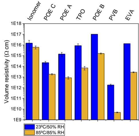
**Figure 4.** Volume resistivity values measured for all the seven encapsulants (after the lamination process) at two different environmental conditions: lab environment (23°C/50% RH) in blue and damp heat (85°C/85% RH) in yellow. All values are averages of five different samples.
