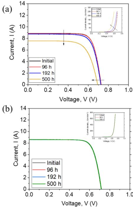
**Figure 3.** One-sun and dark IV curves of G/G mini-modules encapsulated with (a) POE C and (b) EVA and tested at 85°C/85% RH/-1000 V for up to 500 h. We observe that both the one-sun and dark I-V curves remain stable in the case of the mini-module encapsulated with POE, whereas there is a gradual degradation for the mini-modules encapsulated with EVA.
