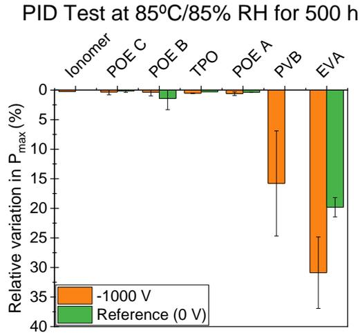
**Figure 1.** Relative variation of the maximum power ( $P_{max}$ ) of SHJ cells encapsulated in a G/G structure with seven different encapsulants, after 500 h of test at 85°C/85% RH and -1000 V and 0 V (as reference) conditions. Values are the averages of each type of samples.
